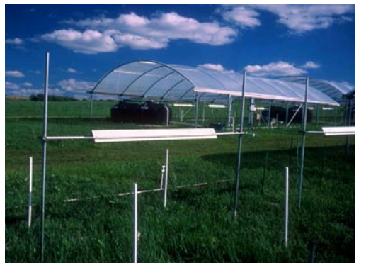
Figure 3. Top: View of one of the Rainfall Manipulation Plots (RaMPs) prior to installing IR lamps. Bottom: IR heating lamps in a reference plot in the foreground. See text for a more detailed description of the shelter design and operation.
