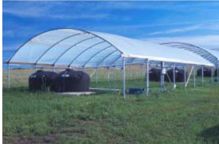
Fig. 27. RaMPs are intact grassland plots beneath fixed-location rainout shelters that exclude and collect natural rainfall, and allow experimental control of the quantity, timing, and variability in rainfall inputs. Shelters (14 x 9 m) consist of clear (UV transparent) poly-ethylene roofs, reservoirs to collect and store rainfall, and an overhead irrigation system. The 6 x 6 m central sampling area has a substantial buffer zone, and 1.2 m deep subsurface barrier limits lateral water movement. For more details see Fay et al. (2000).
