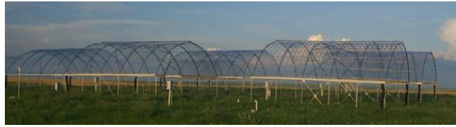
Fig. 4. Passive precipitation reduction shelters at Konza Prairie in an annually burned watershed near 001D.
